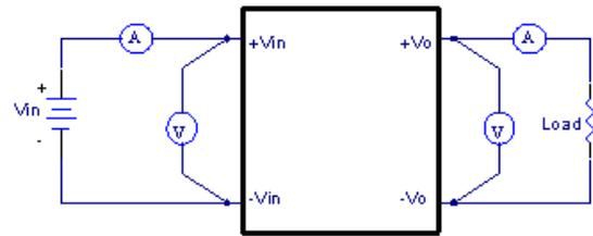
Figure 5 EC3A Series Test Setup
