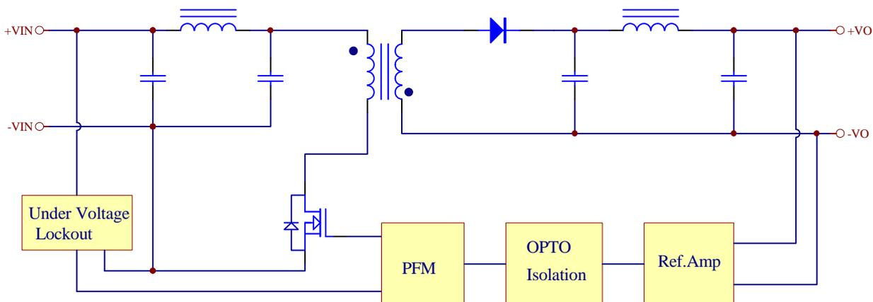
Figure 1 Electrical Block Diagram of single output module
