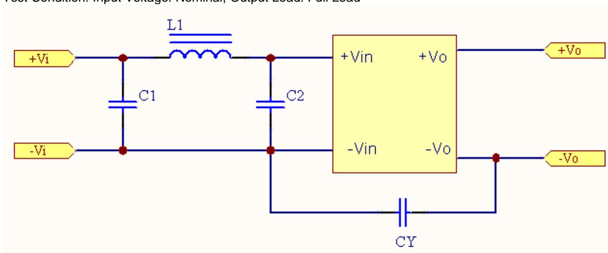
Figure 9 Connection circuit for conducted EMI testing
