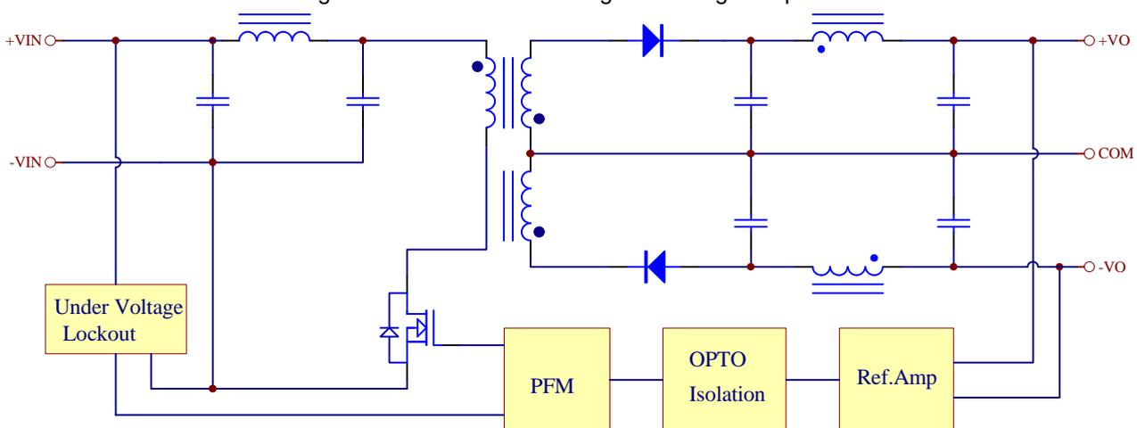
Figure 2 Electrical Block Diagram of dual output module
