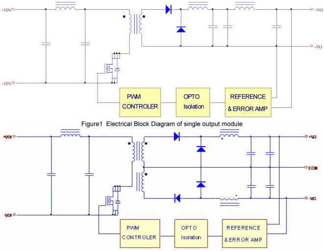
Figure2 Electrical Block Diagram of dual output module
