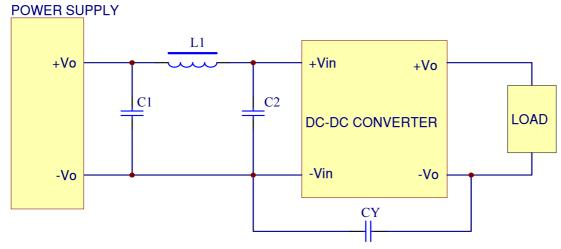
Figure12 Connection circuit for conducted EMI testing
