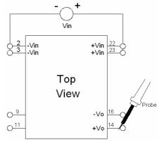
Figure 10 Using Probe to Measure Output Ripple and Noise
