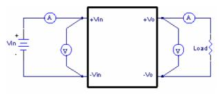
Figure8 EC4AW Series Test Setup
