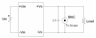
Figure9 Using BNC to Measure Output Ripple and Noise
