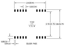
Figure5 Recommended PCB Layout Footprints for SMD packages Lead Free Hot Air Reflow Profile
